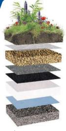
CARLISLE® intensive component green roof system consists of multiple layers including drainage, filter, substrate and a wide range of landscaping options depending on the substrate depth.
