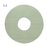
Cut out a sleeve. The outer diameter is the diameter of the passage plus 100 mm. The inner diameter is the diameter of the passage minus 40 mm.
