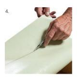
(text by picture 3): Cut the release film across this width with the cutter knife.
