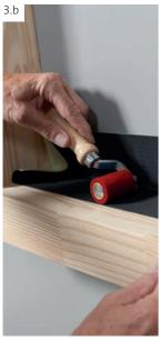
Then press it well with the silicone pressure roller.
