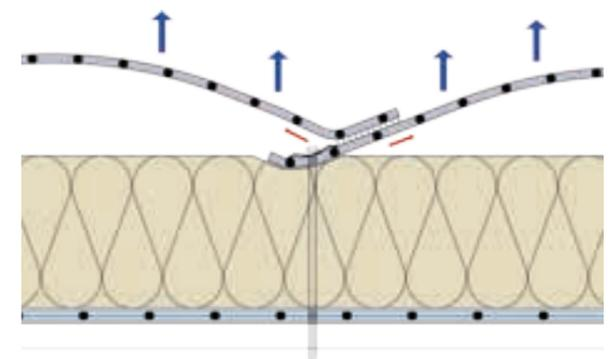
Since the fixing points are distributed like a grid across the entire roof and not just placed on the membrane joints, the wind forces are supported more evenly. As a result, the point load per fixing element is less and the system can handle higher wind forces with fewer fixing requirements.
