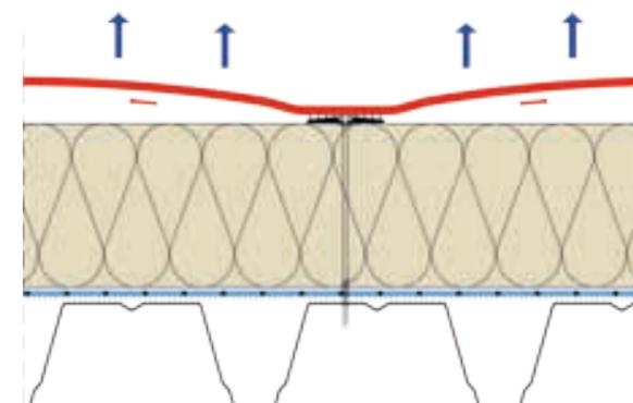
The position of the fastening plate is defined based on the wind load calculations for the property and distributed in the roof system. As a result, despite mechanical fixing, larger membranes can be used and a clear reduction achieved in the seam proportions and seam overlap compared to conventional systems fixed in place by mechanical means.
