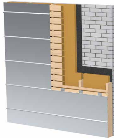
Horizontal standing seam system
