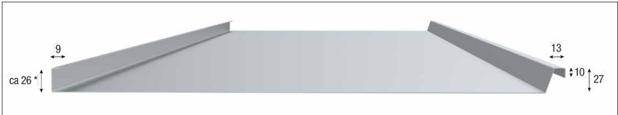
Figure 5.1.2 Dimensions standing seam bay
