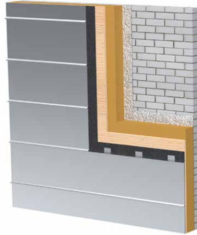
Horizontal standing seam system
