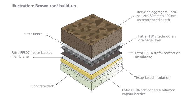
Fatra green roof systems are laid on a bonded Fatra roof. A Fatra Technodren drainage layer is laid over a protective fleece and then covered with a filter layer. The green roof that follows can consist of a mixture of reclaimed site waste and small hardy plants, or can be planted out with sedums, or even small bushes. To ensure that each roof performs as expected Fatra has partnered with a number of green roofing experts to provide detailed design advice and installation services.
