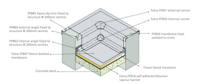
Illustration: Fully adhered parapet and corner detail
