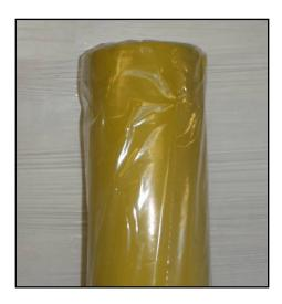
Fatra Polyethylene Vapour Control Layers should be installed on the 'warm' side of the insulated structure, with special care being taken to ensure that all seams and holes are sealed effectively - thus rendering the whole structure moisture vapour proof and improving thermal performance. It is important that Fatra Polyethylene Vapour Control Layers should be continuous in order to prevent vapour entering the wall or the roof.
