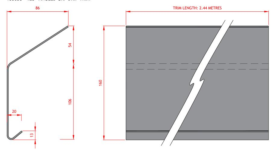
Drip trims are fitted to the perimeter edge of the roof area, where rainwater drains off the roof to a gutter.
