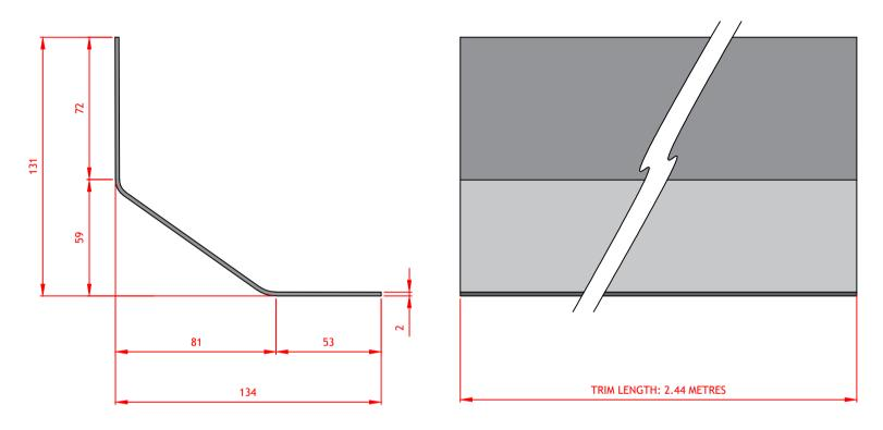
Fillet trims are installed at the junction where an adjoining wall meets the flat roof area. They enable Polyroof waterproofing systems to be dressed effectively through the junction details and assist in the deflection of rainwater.
