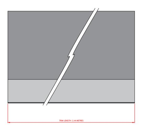
Fillet trims are installed at the junction where an adjoining wall meets the flat roof area. They enable Polyroof waterproofing systems to be dressed effectively through the junction details and assist in the deflection of rainwater.
