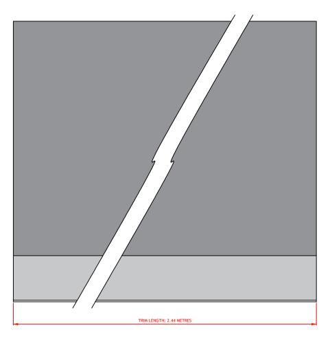
Fillet trims are installed at the junction where an adjoining wall meets the flat roof area. They enable Polyroof waterproofing systems to be dressed effectively through the junction details and assist in the deflection of rainwater.
