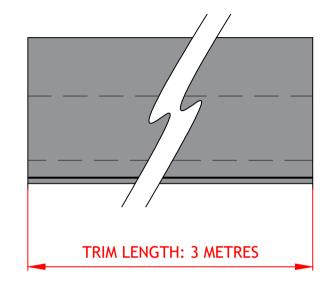
GRP LEAD ROLL Trims can be used to simulate the appearance of lead roll joint details on flat roof areas, for conservation work, and to straddle cables and technical details.
