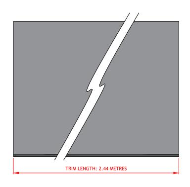
GRP RIGHT ANGLE trims can be used at abutment details where it may not be practicable to use an angle fillet trim, for example at the deck upstand junction of a balcony.
