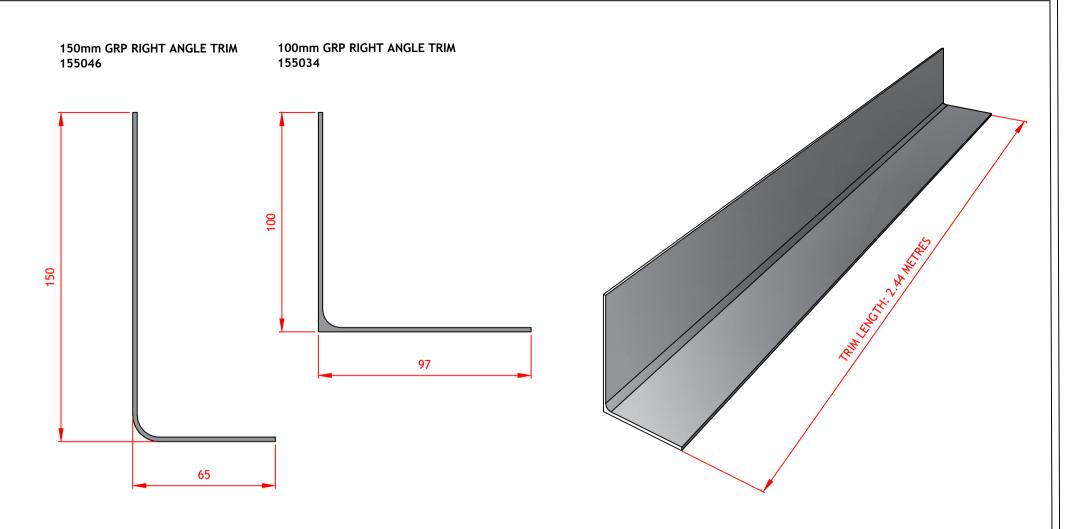
GRP RIGHT ANGLE trims can be used at abutment details where it may not be practicable to use an angle fillet trim, for example at the deck upstand junction of a balcony.
