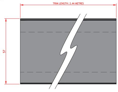
Termination bars are used on an upstand details to seal and protect the termination detail of a Polyroof liquid system, normally where a chase or flashing termination detail can not be utilised.
