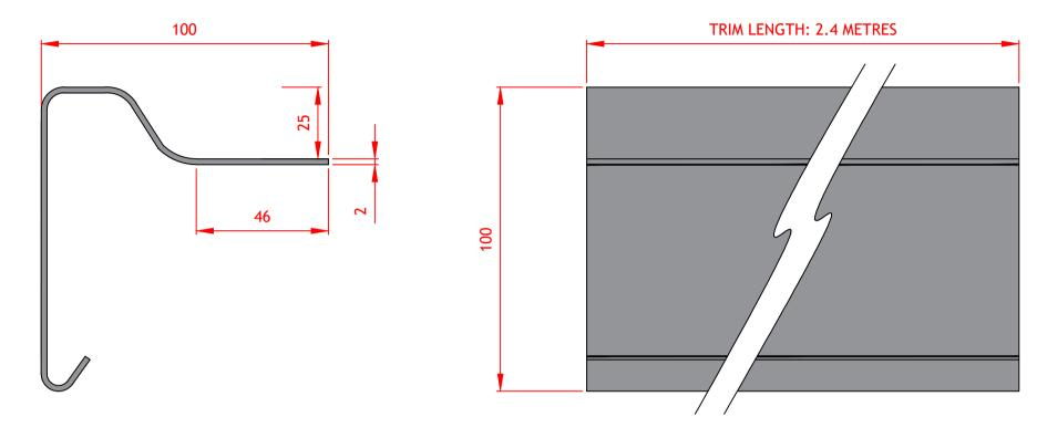
Upstand Fascia Trims are fitted to the perimeter edge of the roof area, where there is a watercheck detail.
