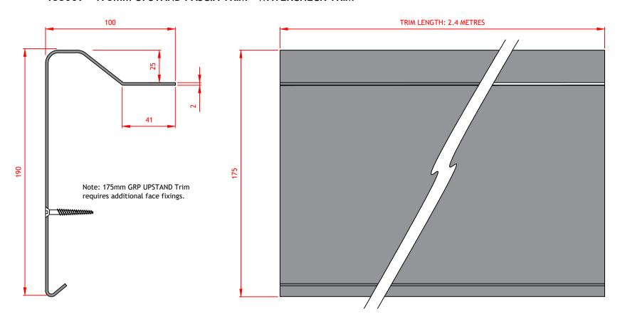
Upstand Fascia Trims are fitted to the perimeter edge of the roof area, where there is a watercheck detail.
