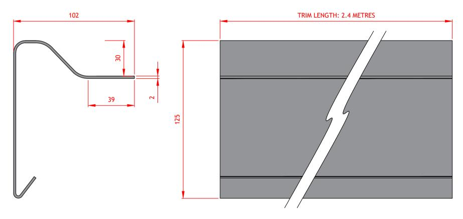
Upstand Fascia Trims are fitted to the perimeter edge of the roof area, where there is a watercheck detail.
