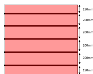
Perimeter Roof Zone 200mm Centres
