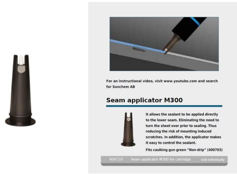
Applicator that guides the <u>Seam Sealant</u> tubes during application to the seam. Reduces the risk of scratches and damage during installation as there is no need to turn the sheet. Easy to control the width of the joint.
