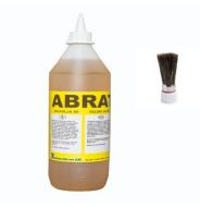
Abratex lap sealing oil is made from non-drying oils and is used as a seam sealant for all types of metal roofs. The lap sealing oil swells on contact with water which happens in the joint. The product must therefore not be diluted. Lap sealing oil is excellent for sheet metal seams or cross-welts. Lap Sealing oil is applied with a twist on brush head.
