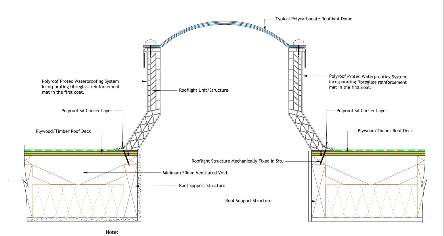
All substrates are to be suitably prepared and primed as required in accordance with the project specification details, prior to the installation of the Polyroof waterproofing system.
