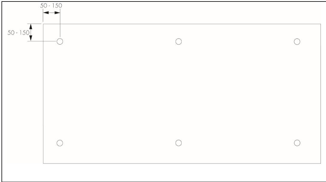
Figure 2 Fixing layout 2400 by 1200 mm board — minimum number of fixings
