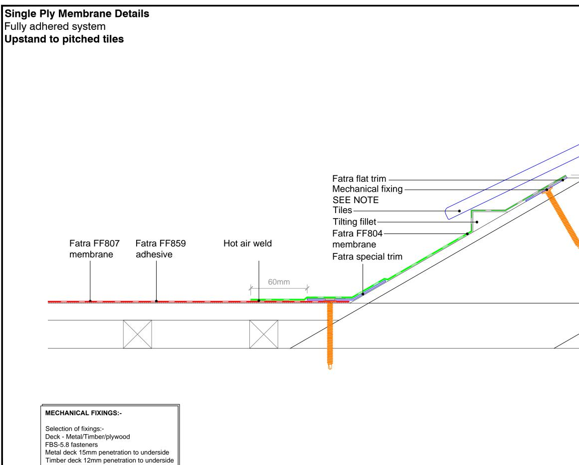
Deck - Concrete FHD-6.1 fasteners
